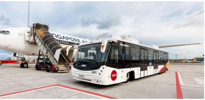
on a single charge. They are constructed using lightweight aluminium frames for the body, aimed at reducing carbon emissions and noise levels. This design improves overall operating cost and efficiency.
